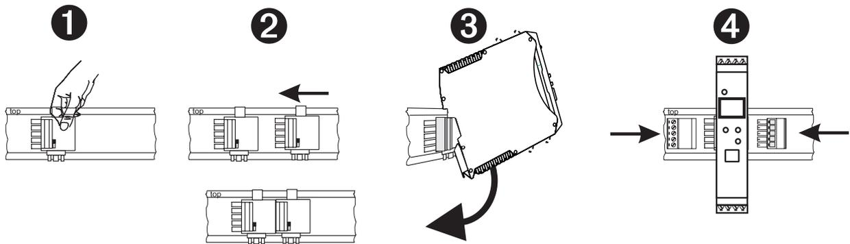
The devices are intended for vertical mounting on 35 mm top-hat rails to EN 50 022.
