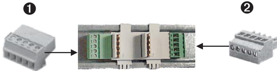
The connectors are fitted with screw terminals with standard 3,81 mm spacing for lead cross sections up to 1,5 mm<sup>2</sup>, and should be tightened with a torque of 0,22 - 0,25 Nm.
